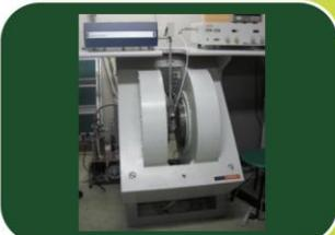
Irradiated samples were measured using the EPR Spectrometer at Okayama University of Science
