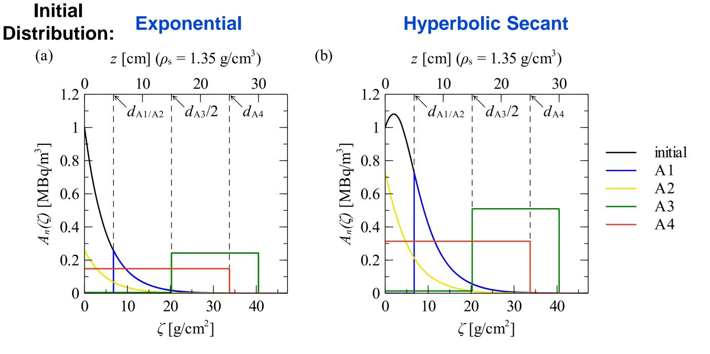
Model for change in radioactivity distribution with depth after remediation
