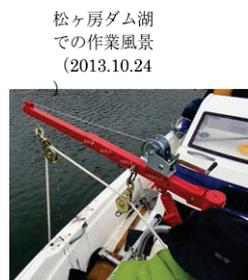
Using core sampler with drop-weight at the deep water point at 2012 and 2013
