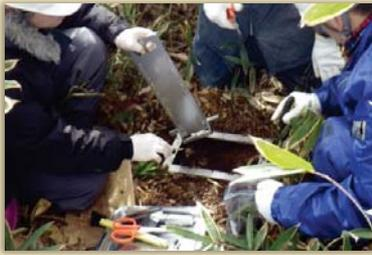
Soil sampling by scraper plate (sampling interval: 1 cm)
