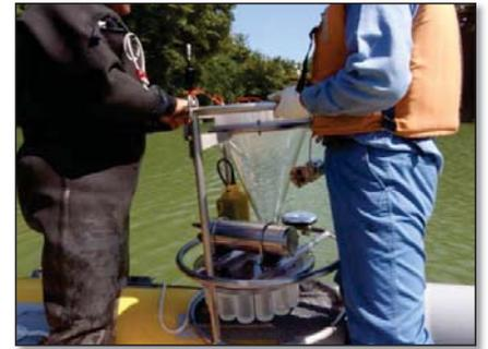
**Sampling of sinking particles**
