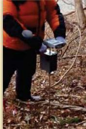
Soil thickness measurement by penetration test
