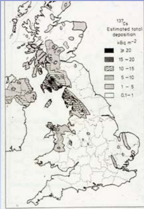
Fig. 2 Estimated total deposition of 137 Cs (kBq m -2 ) over the United Kingdom due to Chernobyl releases, calculated from a washout factor of 6.5 10 -3 , the rainfall data and air concentrations.
