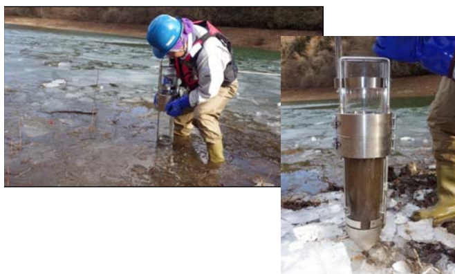
Core logging (undisturbed sampling)
