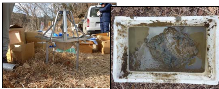
Sampling of bottom sediments (Smith-McIntyre Bottom sampler)
