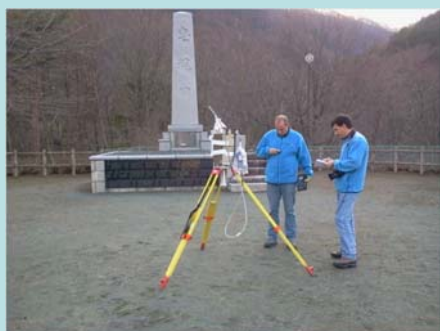
In situ measurement using a portable Ge gamma spectrometer
