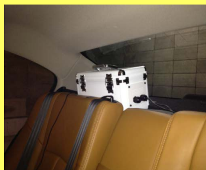
Mobile monitoring with the KURAMA system mounted in cars
