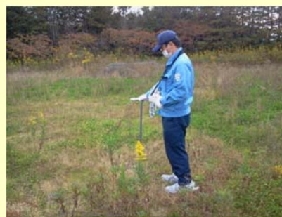
Measurement on ground (undisturbed flat fields) with a survey-meter
