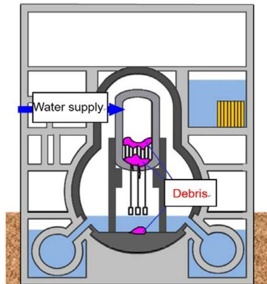
**Reactor containment vessel
