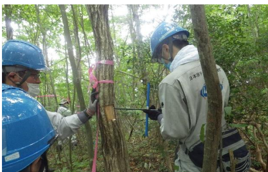
Collecting xylem using an increment borer
