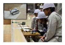
For crawler-type robots, they first tried to operate it while confirming with their own eyes. Then, they operated only by the image taken by the camera loaded on the robot. It was difficult to see the front of the robot due to the extremely narrow scope of the camera. So, the students seemed to struggle because it was hard to operate the robots (see the left photograph). For underwater robots, the students also struggled, because it was difficult to operate
