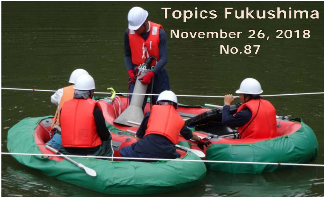
JAEA staff measuring radiation on the reservoir (instrument seen in the center is the radiation detector).
