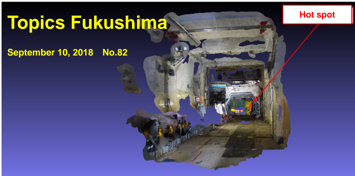
Figure 1. Reactor building reproduced in a virtual space. The high-radiation part (hot spot) is shown in red.
