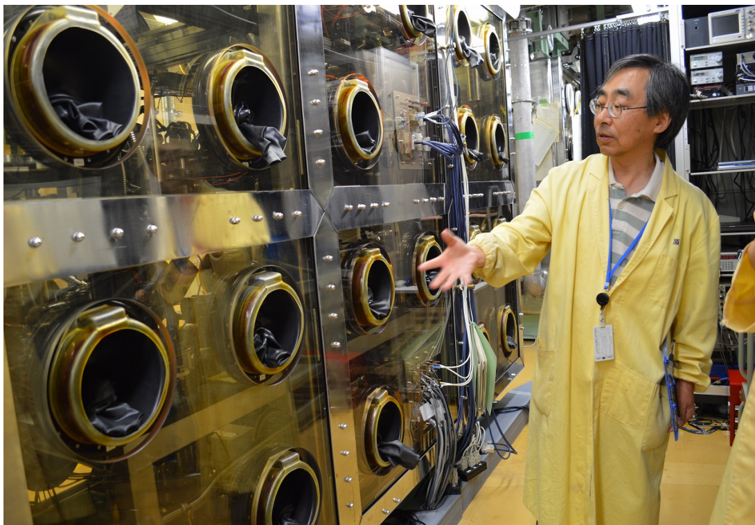
The glovebox was repaired for laser spectroscopy experiment by newly installing windows for laser and terminals for optical fibers.
