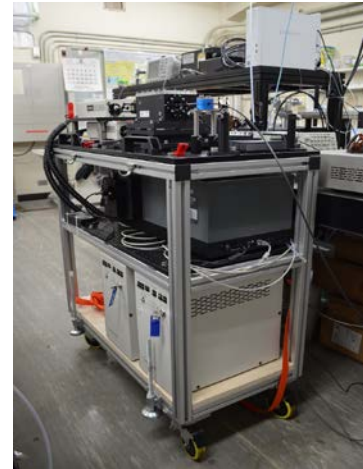
Prototype of portable Laser-Induced Breakdown Spectroscopy (LIBS) instrument with fiber transmission that can be used in water
