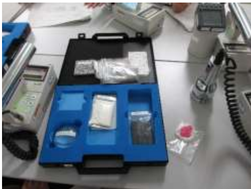
Samples used for learning radiation measurements and characteristics of radiation (kombu, granite, chemical fertilizer, mantle, etc.), and radiation-shielding material (steel plate)
