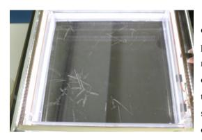
Next, the students experienced the observation of radiation with cloud chamber, and practiced the radiation measurement using radiation detectors. Using a cloud chamber, tracks of radiation (lines produced by radiation like vapor trail) can be observed without using radiation source (left photo). The students learned by the observation that there are natural radiation and
