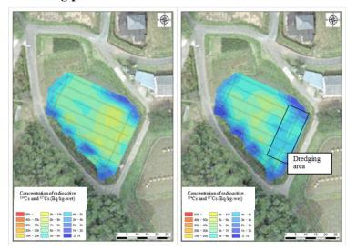
Example of radioactivity measurements before and after dredging. Left figure: before dredging. **Right figure: after** dredging. The maps were made based on the data measured with the p-Scanner at five-meter intervals. Values between measuring points were interpolated by the use of commercial GIS (geographical information system) software.
