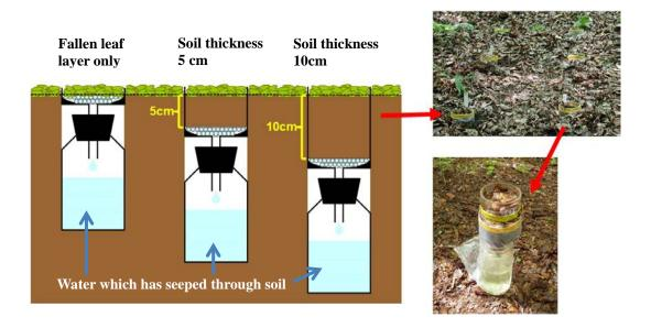
Lysimeters are used to collect water which has seeped through soil
