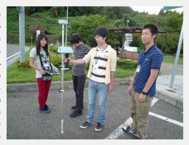
vegetation or turf exhibited a slightly higher dose than the parking lot paved with asphalt. Also, the interlocking blocks under the rainwater drain pipe exhibited a higher dose than other locations. Such facts can be understood visually by using the  $\gamma$ -plotter. In addition, the students found that values differ, even at the same location, depending on the type of measuring device, and learned how to use measuring devices and points to consider regarding measurement.
