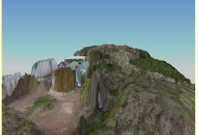
←3D topographical map developed by ortho-images
