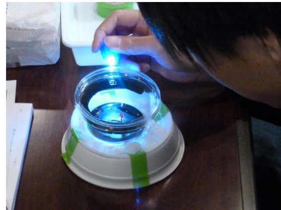
The picture above shows the participants observing radiation using a cloud chamber. The chamber is full of alcohol vapor and cooled. When the radiation passes through, the vapor collects along the path forming a white "cloud" on the path. The picture below shows the cloud chamber fabricated by the participants using familiar
