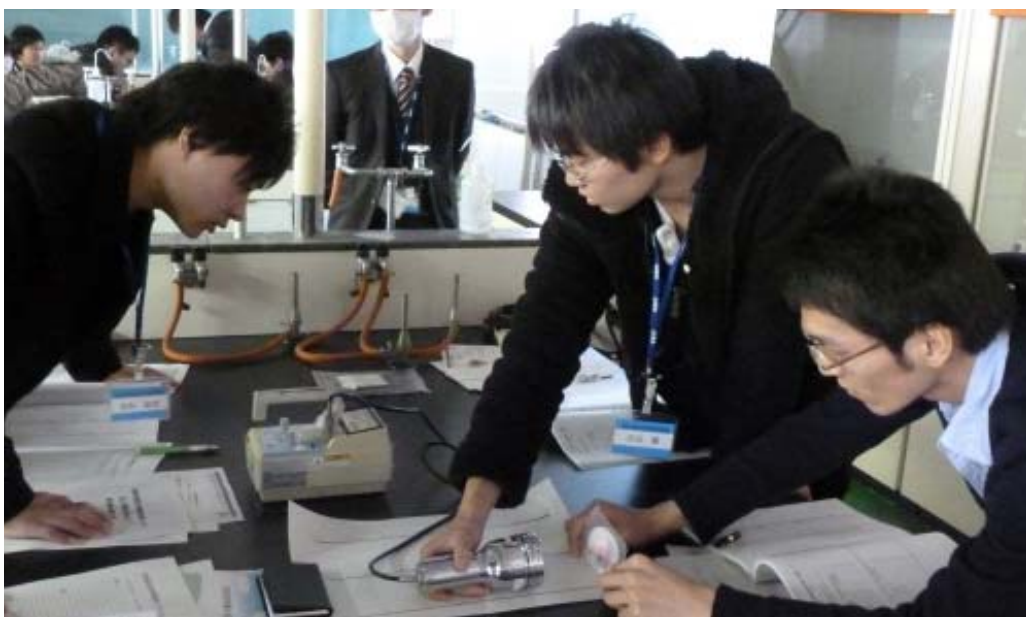
Amount of radioactivity (Bq) of a mantle is checked with a GM survey meter. You can see that the dose rate goes down as you move away from the radiation source (left).
