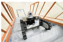
▲Mock-up stairs can simulate the stairs in the reactor building of 1F
