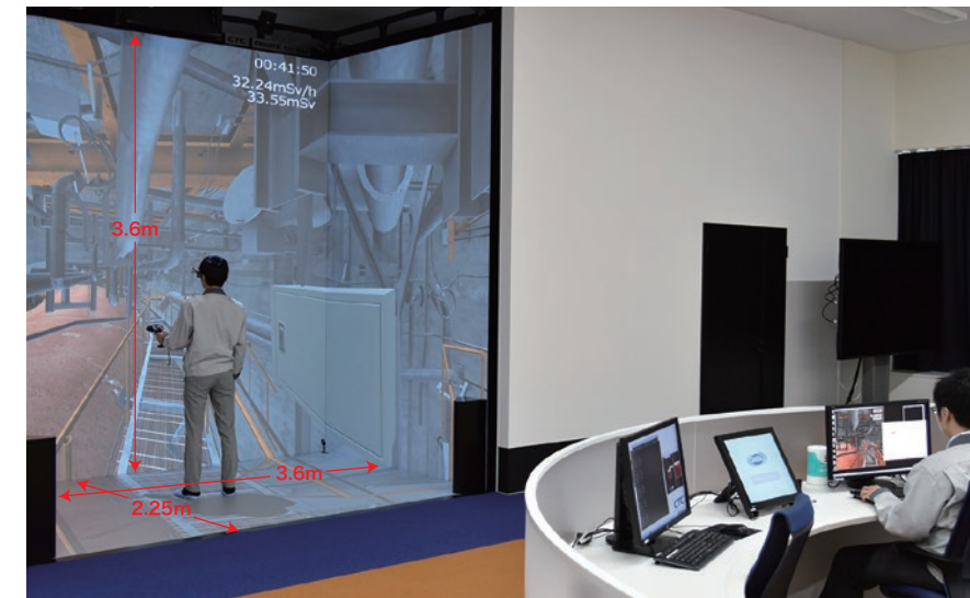
▲VR system that enables to project various types of 3D data on the front, right, left and bottom sides of a cubic screen.
