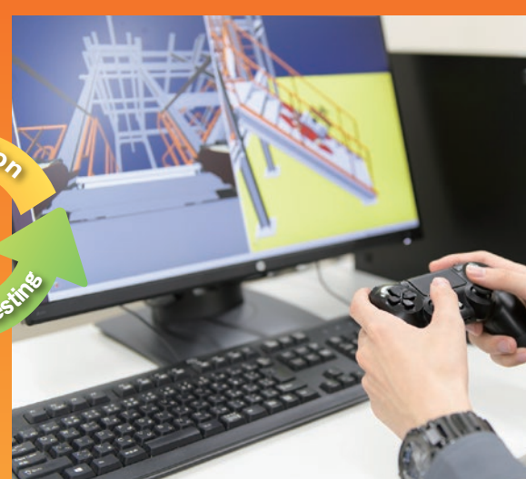
Remote control training with a robot model in a virtual decommissioning environment built inside a computer
