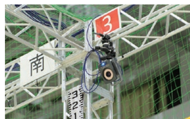
▲High-speed cameras provide an overall picture of movement from all directions.
