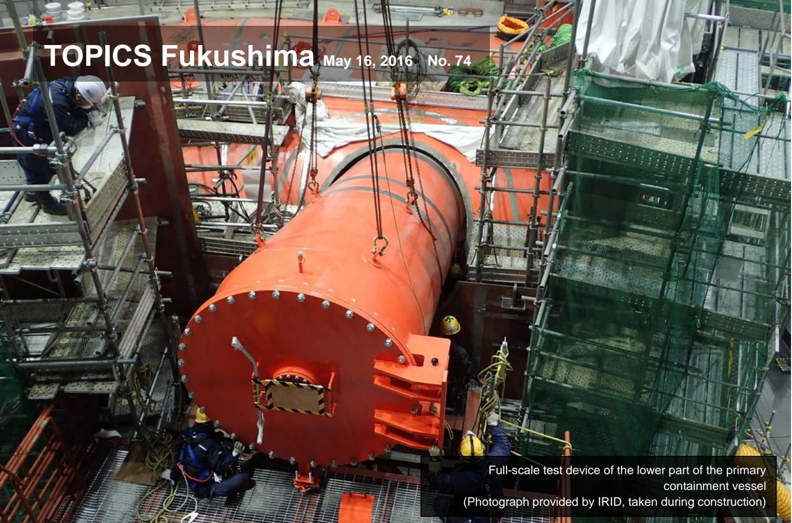
Full-scale test device of the lower part of the primary containment vessel
